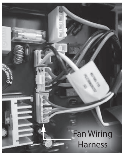
Figure 129 - Locate fan wiring harness on control board
