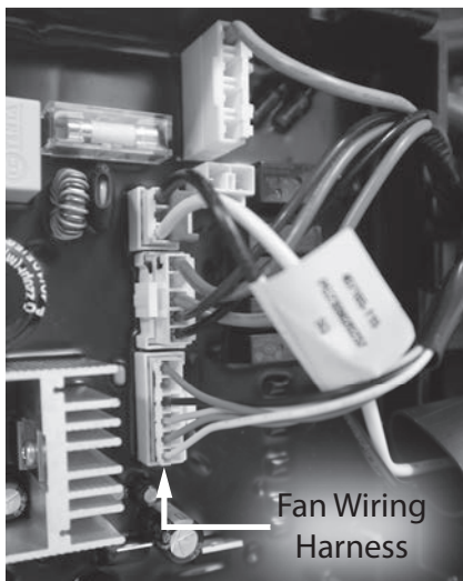
Figure 110 - Locate fan wiring harness on control board
