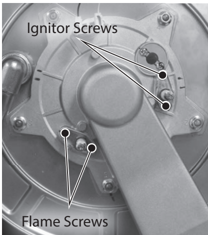
Figure 116 - Remove ignitor rod and flame sensor screws
