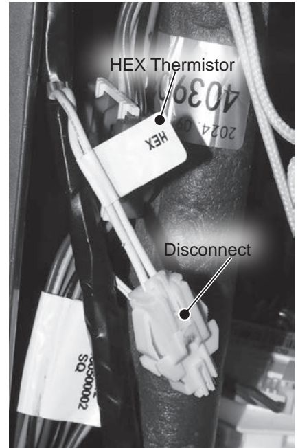
Figure 43 - Disconnecting HEX thermistor
