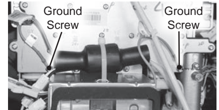
Figure 109 - Removing green ground wires
