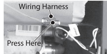
Figure 64 - Wiring harness location
